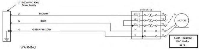
Do not route auxiliary contact cable in the same conduit as motor cable
