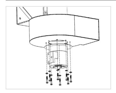
STEP 2. Attach capture arm to swivel base.
