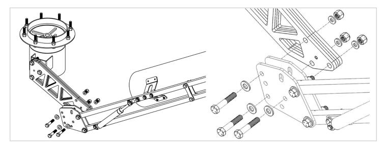
STEP 6. Attach Capture Arm to Swivel Base. (J-Bracket)
