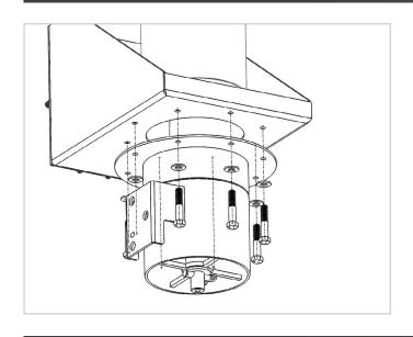
STEP 7. Attach capture arm to swivel base.
