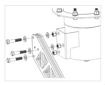
STEP 8. Attach J-Bracket to Arm Swivel.
