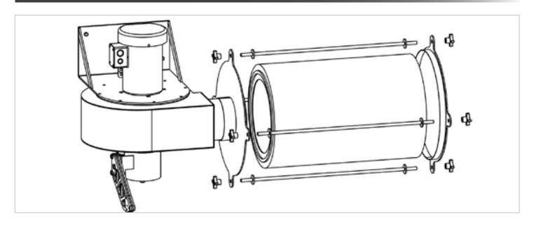
STEP 4. Attach Filter to Blower Assembly
