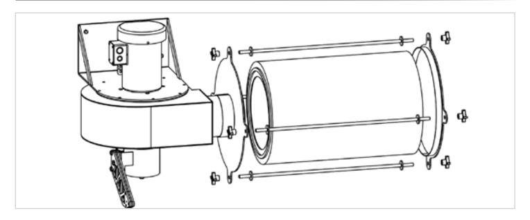
STEP 5. Attach Filter to Blower Assembly
