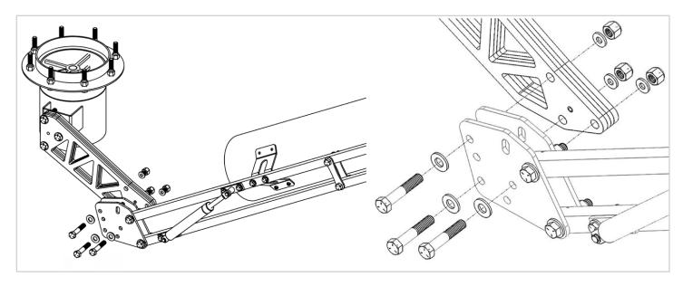
STEP 9. Attach Capture Arm to Swivel Base. (J-Bracket)
